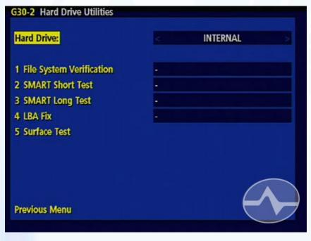
The Advanced Tests Menu lets you run a lot of very specific tests. It also allows you to run some very deep tests on your hard drive, as well as testing your receiver's abilities to use front panel buttons, the remote, and even check your network and satellite connections.
