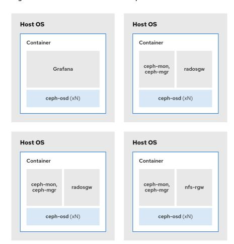
The diagrams below shows the differences between storage clusters with colocated and non-colocated daemons.
