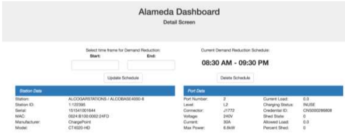
Figure 11: Smart Charging Control System Dashboard for Fleet Electric Vehicles and Direct Current Fast Charger
