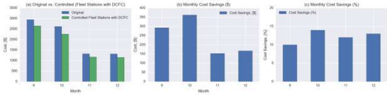
Figure 43: Cost Savings Considering Only Smart Charged Direct Current Fast Charging Sessions at AICoPark Garage in September-December 2017
