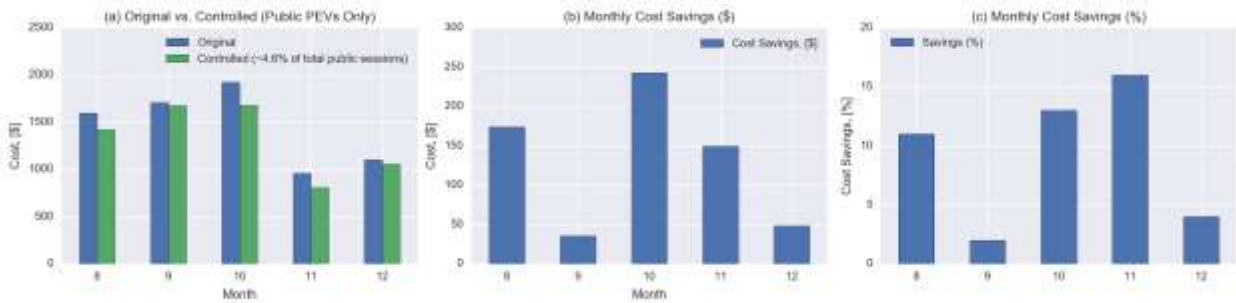
Figure 42: Cost Savings Considering Only Smart Charged Public Sessions at AICoPark Garage in August-December 2017
